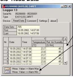
If there are logger data in the memory they can be read out (menu 'logger – read out logger data') and be viewed in form of a table.
