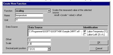
The source is a logger window with data in the unit [°C], which has to be opened before calling up the input
