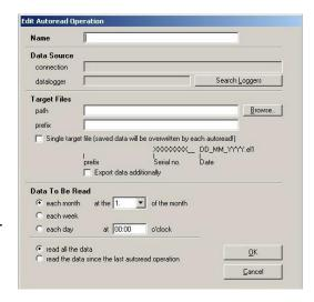
This file wile be saved after the autoread automatically in the previously entered path. The data to be read in can be adjusted to Your needs.
