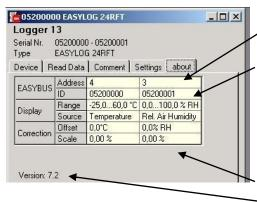
Display of all the remaining properties and settings of the logger. **EASYBus -Address:** cannot be changed via GSOFT40K. To do so please use our EASYBus-Configurator software. Display data
