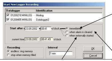
**Start when externally started:** the logger recording will only be started externally, even if the time set has been reached. An external start can be carried out on site with the help of the ,EBSK-1' starting key.
