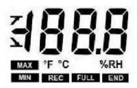
°C.. Temperature in degrees Celsius °F.. Temperature in degrees Fahrenheit %RH..... Relative humidity (KH 50)
