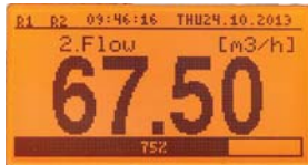
The current value of the measurement signal Height of the digits: 18 mm
