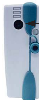
Jack 3.5 connector Input for KISTOCK-PC software
