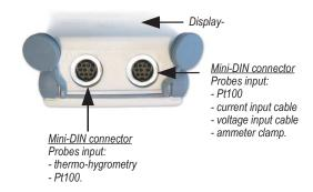
Only Class 300 probes shall be connected (not any other probes), as described above.
